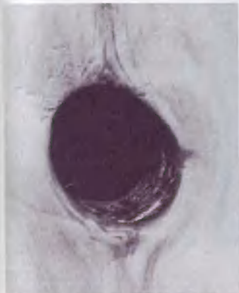
Knot holes: Caused by wood growing around a dead branch.
